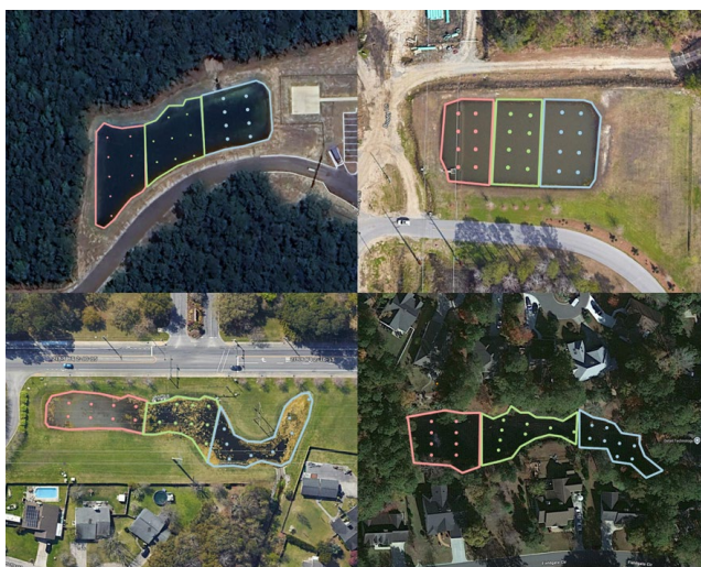
Figure 1. Ponds with an example grid point design to randomly select sampling locations. The blue section represents the inlet, green represents the middle, and red represents the outlet. Maps created in QGIS.
